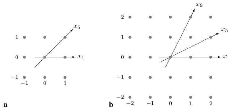
Fig. 6 Forming the coordinate systems in a given pixel (0,0) using its neighbourhoods: (a) 1<sup>st</sup> order – pixels at distances from 0.5 to 1.5; (b) 2<sup>nd</sup> order – distances from 1.5 to 2.5. Only the  $O_x$  axes determined by the given neighbour for the first one of four systems defined by this pixel are marked; the following three systems emerge by rotating this first one by  $\pi/2$ ,  $\pi$  and  $3\pi/2$
