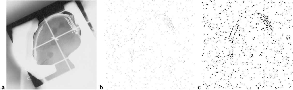
Fig. 8 Example images  $500 \times 500$  for the image registration test. (a) Source image – edges of bony structures selected for registration marked with white pixels; (b) reference image received from image a by translating the selected edges 3 pixels left, 2 pixels down and rotating by  $4^\circ$ ; (c) overlaid image received from a by rotating by  $-1^\circ$ , enhanced for visualisation by replacing each pixel with 4 pixels. Images b, c contain  $\zeta = 0.8$  of outliers
